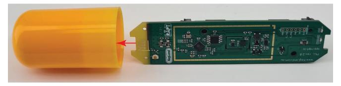
Once the circuit board has been inserted into the yellow housing, screw the two housings together hand-tight until both o-rings are hidden to ensure formation of a hermetic seal.
