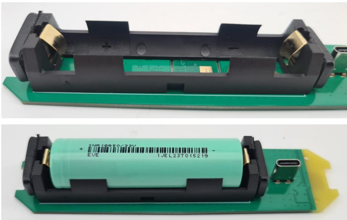
**Important: Incorrect battery orientation can damage the circuit board. This will not be covered by warranty.**
