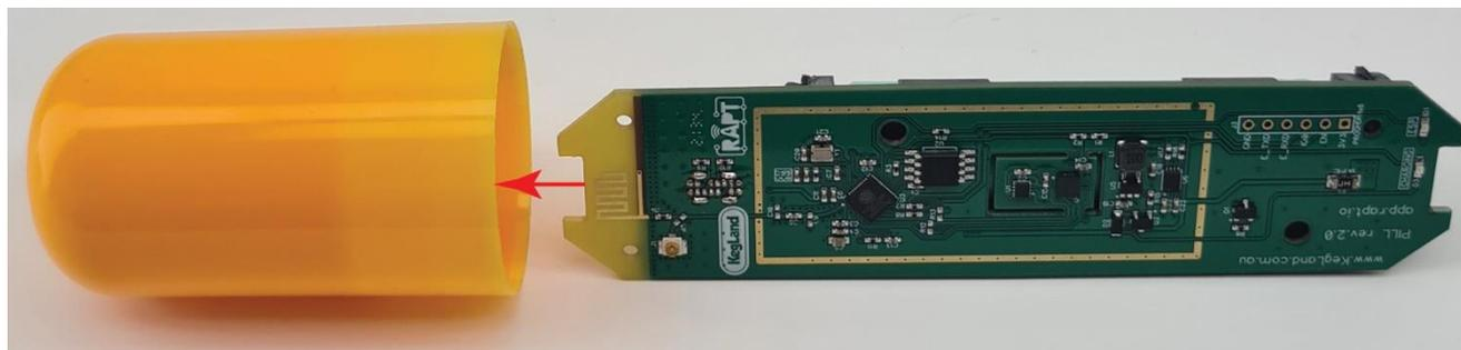
Once the circuit board has been inserted into the yellow housing, screw the two housings together hand-tight until both o-rings are hidden to ensure formation of a hermetic seal.
